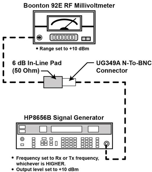
**Figure 5-18 Verify UHF Duplexer Insertion Loss — Connecting Duplexer Cable Assembly**
