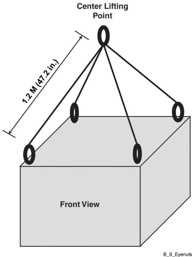
If eyenuts are removed or become loose, install them properly before lifting the equipment rack. Tighten the eyenuts and bolt assembly by hand. Correct eyenut tightness and alignment are crucial to ensure the eyenut assembly performs to its intended lifting capacity. The eyenuts must be aligned to point towards the center lifting point of the cabinet and tightened to between 90 to 120 in-lbs torque.
