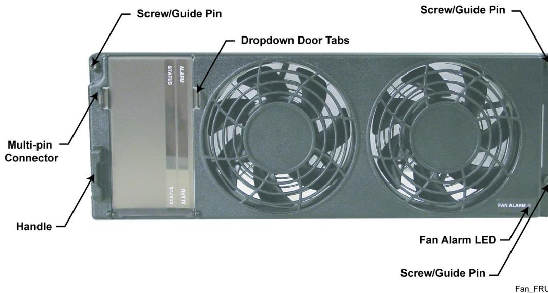
The fan module has one Fan Alarm LED visible on the lower right corner of its front panel. The Alarm is red during Lamp Test (for a second or less), and remains red if there is a fan failure. A fan failure alarm occurs if the built-in speed sensor detects if either fan drops 30% below rated speed. A red Fan Alarm indicates that the fan module must be replaced.
