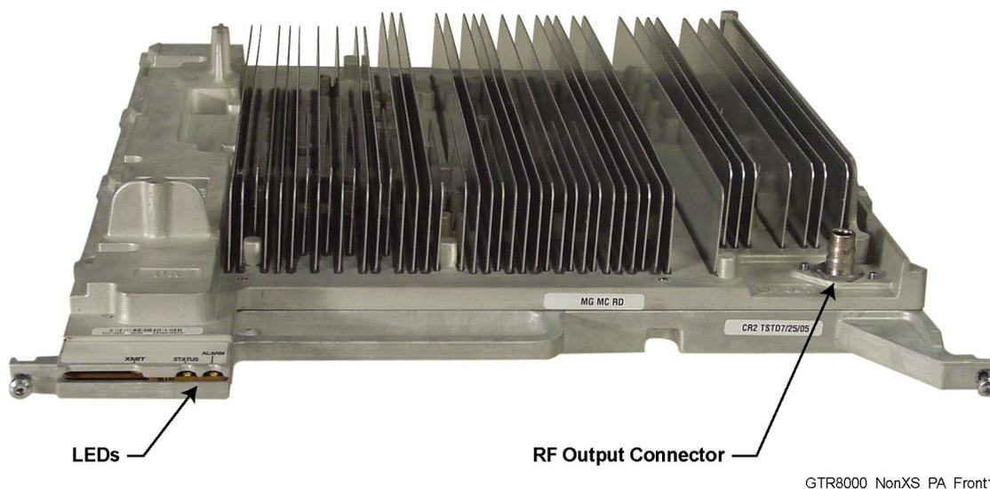
The power amplifier is comprised of six internal modules:
