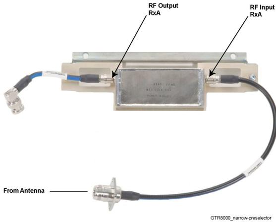
**Figure 9-13 Preselector Filter (UHF)**
