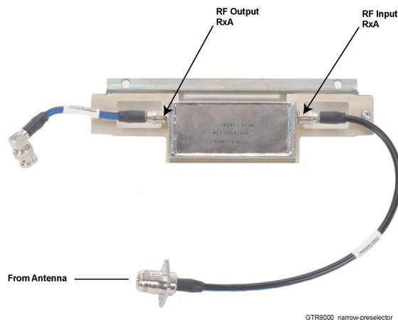
The preselector provides a first level of band pass filtering for inbound RF signals. RF input and output connectors are cabled to the GTR 8000 Base Radios RF Output RxA. This filter must be included to fulfill TIA102-CAAB Class A spurious response rejection (90 dB). The filter is usually not required when using a receiver multicoupler system. This filter can NOT be retuned in the field.
